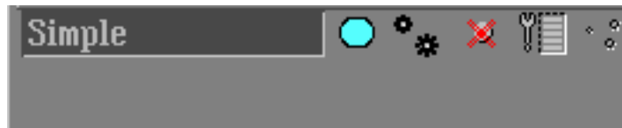
Fig. 9. Panel of objects. From the left to the right: field with object name, button of object visualization in the scene, button of model activity, button for deleting the object from scene, button to call panel with object properties, button of visualization of inclusions (last button is workable after creating of object inclusions ).
