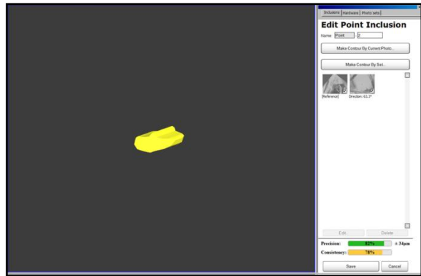
Final model of inclusion created by intersection of two cylinders obtained with two different photos, zoom 50x (M-Box MZ 16A)
